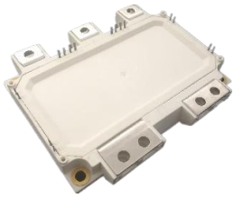
A1: 3 phase bridge/double copper
